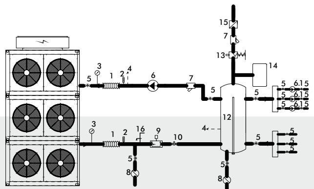
Example with internal loop pump and external zone pumps
